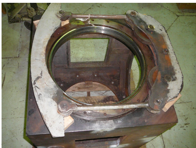
The Declination Axis Main Bearing Polar Load Relief Assembly, sitting roughly where it belongs on the Cube
