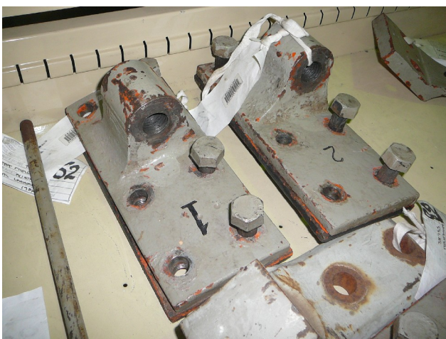
Tube lugs, with very old paint, for attaching the mirror cell to the lower end of the optical tube
