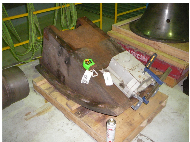
The Quadrant, which holds the lower polar axis bearing that takes much of the 8-ton moving mass
