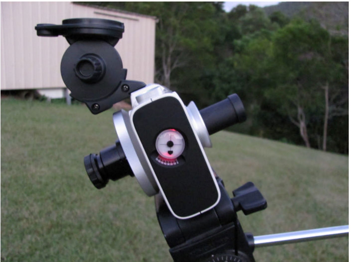
Above: Vixen Polarie fitted with optional polar scope and polar meter which slips into the hot shoe adaptor at top of the star tracker. Tilt meter on the side indicates correct elevation corresponding to the users observing latitude.
