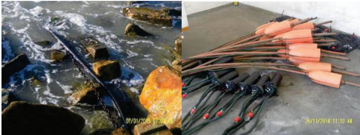
Figure 2-1 Shark Repellent Cable. Left: cable leaving shoreline, Right: cable floats and controls. Source: Jeremy Cliff.
