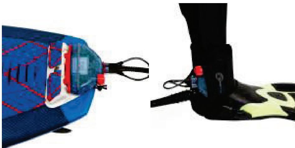
Figure 2-6 Shark Shield devices. Left: surfboard device fitted to rear of the board. Right: attached around the leg of a snorkeler. Source: Lindsay Lyon.
