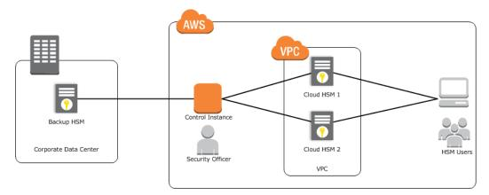
HA allows multiple HSMs to be grouped together to form one virtual device, or logical unit, as seen from the client, similar to clustering or RAID technologies. In an HA configuration, service is maintained even if one or more HSMs are unavailable. For example, if three HSMs are combined into an HA group, service is maintained even if two HSMs are offline.
