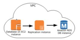
The VPC security group used in this configuration must allow ingress on the database port from the replication instance. You can do this by either ensuring that the security group used by the replication instance has ingress to the endpoints, or by explicitly allowing the private IP address of the replication instance.
