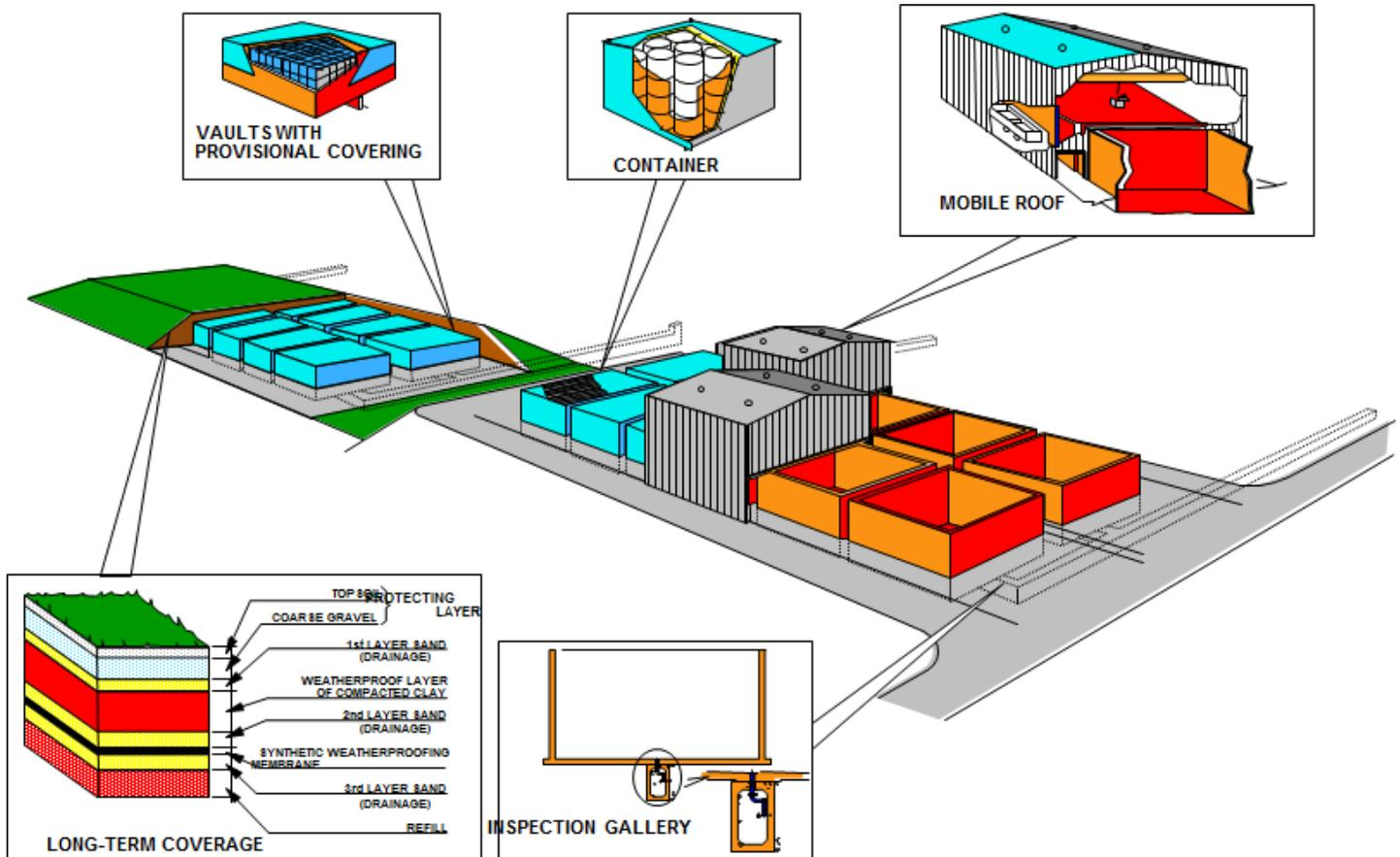
Figure 4.1 : El Cabril LLWR disposal facility, illustrative concept (source: ENRESA, 2015).
