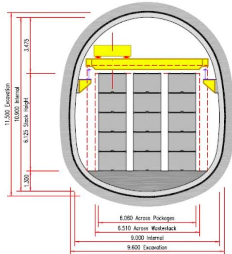
Larger caverns provide flexibility to handle a range of package dimensions. We assume that the operators would define a standard set of package sizes that could be suitable for all potential users.
