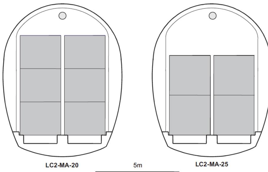
Figure 2.8 : Cross-section of the UK concept for a vault in lower strength sedimentary rocks to contain unshielded ILW packages. The waste packages would be emplaced by overhead crane. (Source: NDA, 2010).
