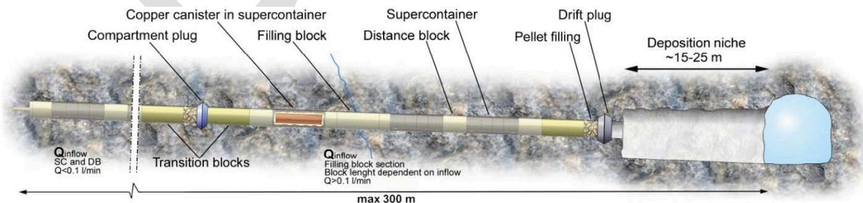
It can be seen from Figure 2.4 that disposal holes are 100 to 300 m long, with supercontainers separated by about 3 – 5 m with bentonite distance blocks. Longer holes can have plugs at intervals and an end plug isolates each disposal hole from the access tunnel from which it is constructed and operated. Emplacement boreholes
