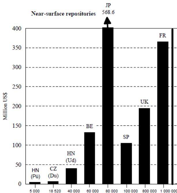
Figure 4.6 : Benchmark operating costs for operating and planned near surface LLW repositories (\$USD per m3), OECD 1999
