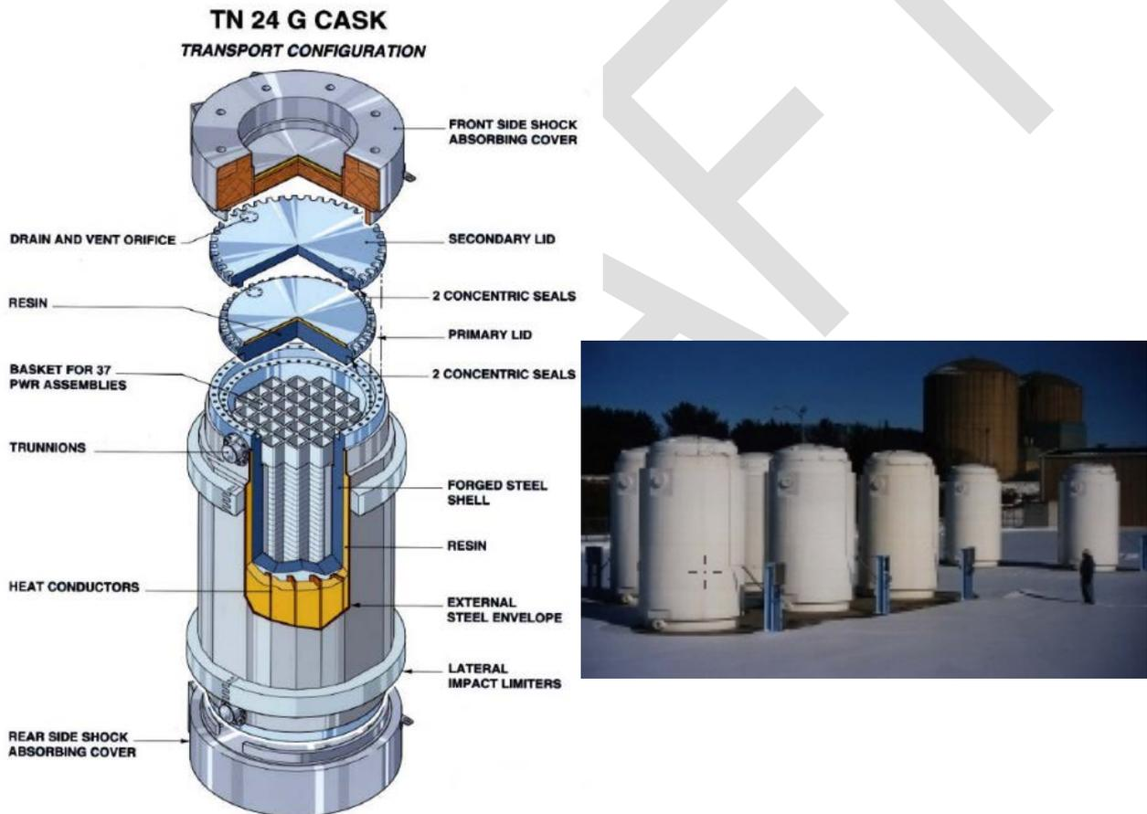
Figure 3.2 (below) shows TN 24 and TN97L casks in robust storage buildings at Doel in Belgium and ZWILAG in Switzerland respectively (Approachv, et al. 1999).
