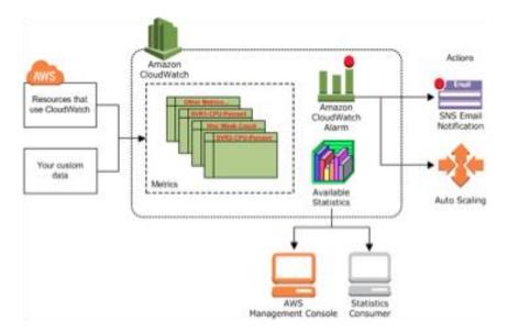
Figure 10: Monitoring Using Amazon CloudWatch
