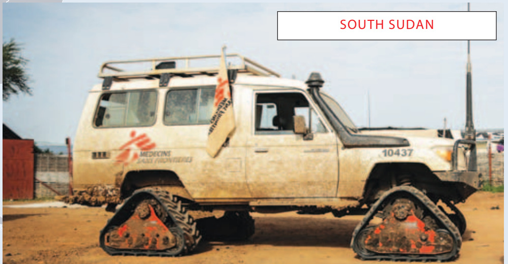
With many roads becoming impassable during the rainy season, MSF teams in Agok have come up with a novel solution to ensure they can continue to reach remote communities: fitting MSF Land Cruisers with specially designed tracks. Photograph © Pierre-Yves Bernard/MSF
