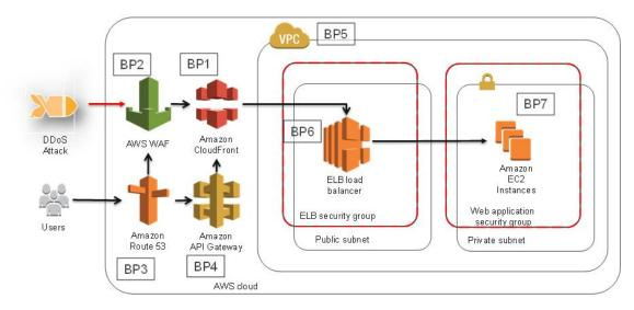
Figure 5: DDoS-resilient reference architecture
