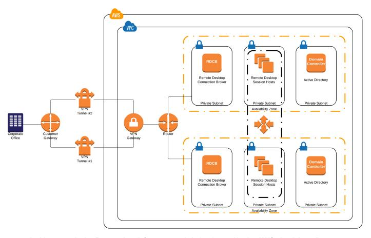
In this scenario the RemoteApp infrastructure is being hosted in the AWS cloud, but all connectivity to and from the AWS cloud is routed over a site-to-site VPN connection.
