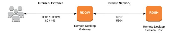
A Remote Desktop Gateway (RD Gateway) server is a type of gateway that enables authorized users to connect to remote computers on a corporate network from any computer that has an Internet connection. RD Gateway uses the Remote Desktop Protocol (RDP) along with the HTTPS protocol to help create a more secure, encrypted connection.
