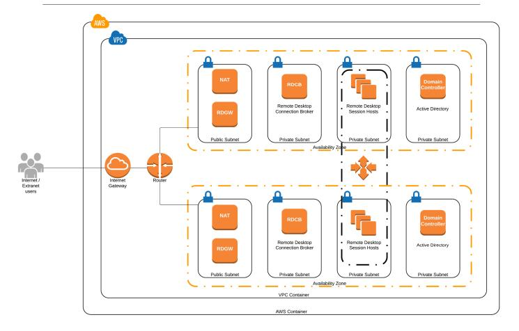
This second deployment pattern is similar in many respects to the previous example. The significant difference is that now the RemoteApp deployment is exposed to public networks.
