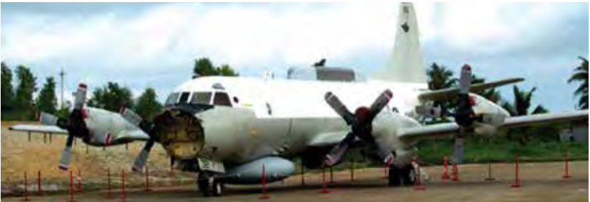
The damaged U.S. Navy EP-3 Reconnaissance plane in Chinese custody on Hainan Island. Visible are the cavity exposed by the missing nose cone, and the broken propeller of the number 1 engine (far right, above). The disassembled aircraft was eventually released to the U.S. Navy for repairs and refitting.
