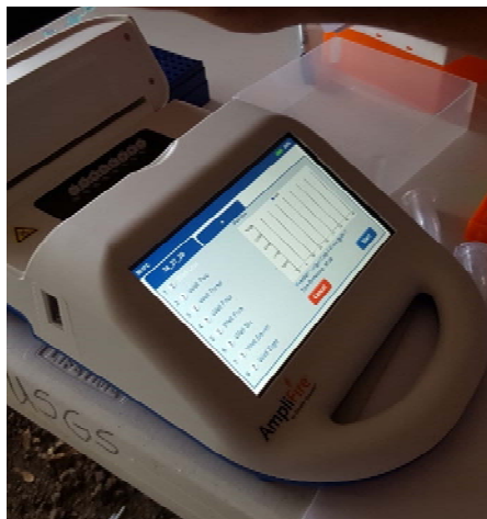
Portable analyzer that provides results of eDNA testing for Asian carp in less than an hour. Possible applications include aiding law enforcement officers and testing of baitfish.
