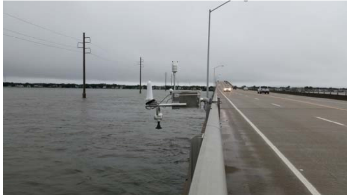
In October 2015, a rapid deployable streamgage positioned on a bridge before Hurricane Joaquin makes impact.
