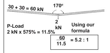
**Note:** The ultimate safety factor will be lowest of all the individual components--the weakest link so-to-speak. But here is a way to determine a not so intuitive elusive link that is not always obvious. If you're not sure of the angle, get a goniometer.
