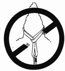
Water Knot (Ring Bend)
