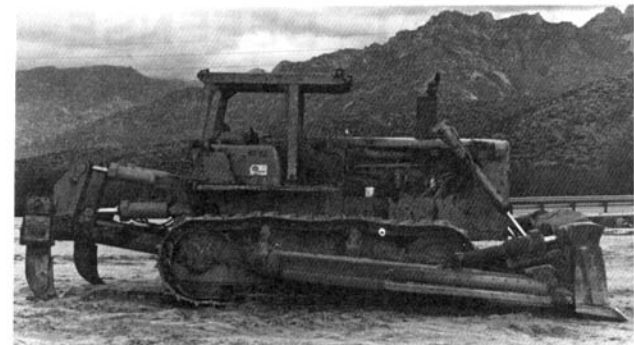
Bulldozer. Note the smoke stack (exhaust pipe).
