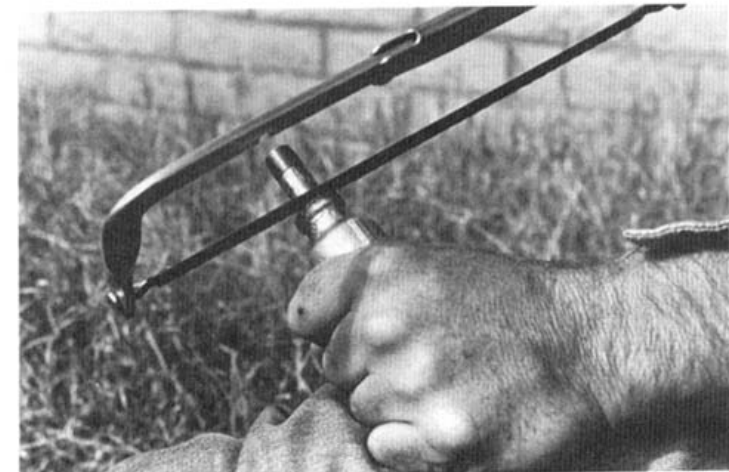
Finally, saw off the 1/4 inch nipple flush with the reducer. Your road spike driver is ready for use.
