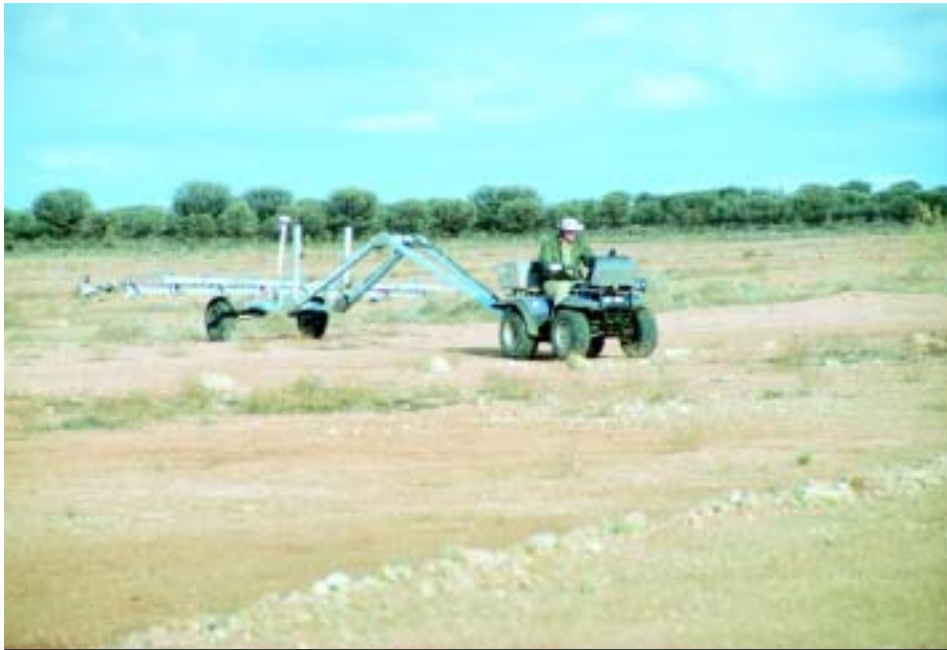
Figure 4.22 Magnetometer survey equipment in use at the TM site.
