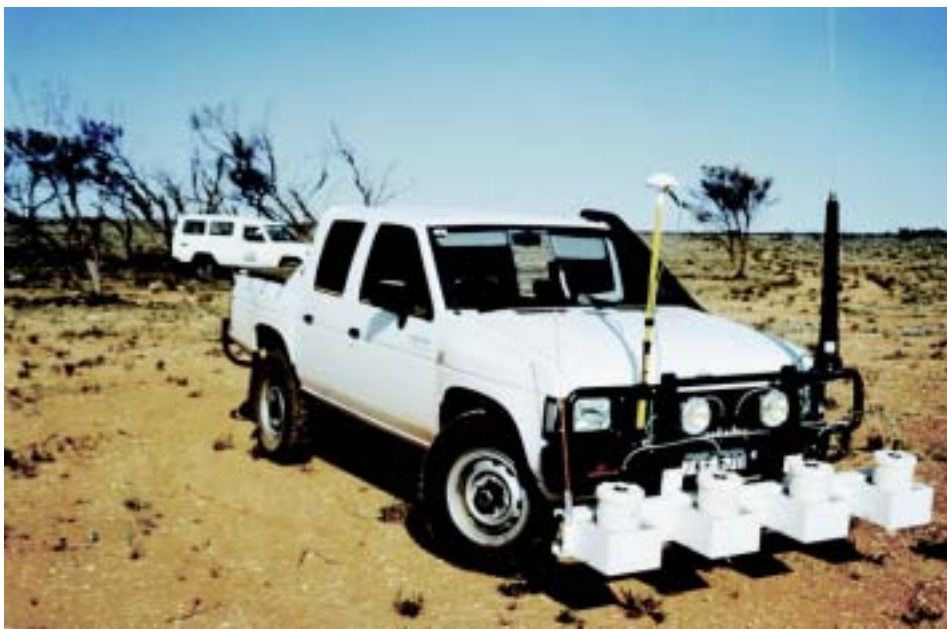
Figure 4.4 The Nissan measurement system—a Nissan vehicle with four sodium iodide detectors for particle detection.
