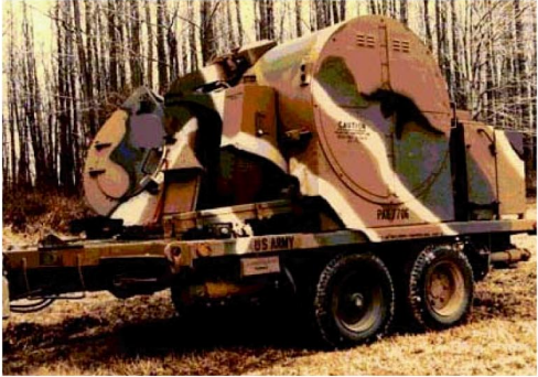
GEMSS (M-128 Ground Emplaced Mine Scattering System) dispenses 800 M-74 antipersonnel and M-75 antitank submunition land mines.
