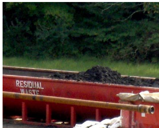
Drill cuttings at a gas well site in West Virginia. Photo by Bill Hughes.
