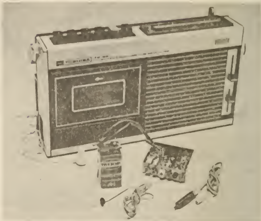
New Scientist's bugging equipment. Standard FM radio receiver with the transmitter and batteries in front. In front of the transmitter are the aerial (left) and microphone (right).
