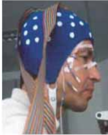
Figure 4.1: A network of 128 electrodes used to map the spatial distribution of EEG signatures around the skull. From reference [49].
