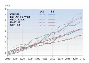
The 10 lines show air temperatures for the region from 60°N to the pole as projected by each of the five ACIA global climate models using two different emissions scenarios. The projections remain similar through about 2040, showing about a 2°C temperature rise, but then diverge, showing increases from around 4° to over 7°C by 2100.
