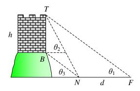
**Figure 7:** To calculate the height h of a building on a hilltop, we need to measure the distance d from the two points N, F at ground level from which we are to take the angles  $\theta$  to the top T and base *B* of the building.
