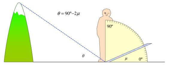
**Figure 8:** Angles must be taken from the ground, for which purpose you might like to tilt a mirror until the reflected mountaintop touches the ground at your feet under the plummet line of sight. Only bear in mind that, because mirrors are whimsical little things, the angle  $\theta$  to the mountaintop is 90° minus twice the tilt  $\mu$  of the mirror.
