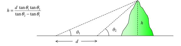
Figure 1: finding the height h of a mountain requires taking three measurements: the distance d between two level points that lie in a straight line from the mountain, and the angles  $\theta$  from these points to the mountaintop.
