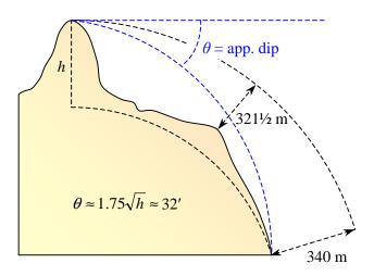
**Figure 4:** Biruni's method leads to results infected by ray bending. Yet, provided you allow for this and take precise measurements, it certainly yields the earth's radius!<sup>1</sup>
