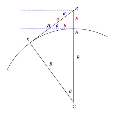
Figure 2: Biruni realized that the figure linking the earth's centre C, the mountaintop B, and the (sea or flat enough) horizon S was a huge right triangle on which the law of sines could be made to yield the earth's radius!
