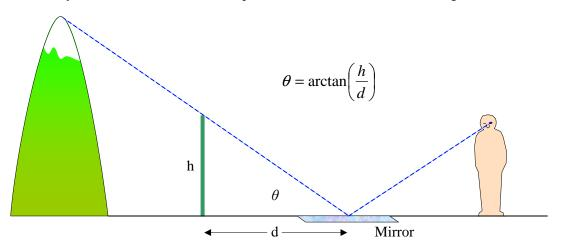
**Figure 9:** An alternative method of finding the angle  $\theta$  from a point on the ground to a hilltop makes use of a mirror on the ground and a stick lined up with the reflected hilltop.<sup>1</sup> This method was first described in Euclid's *Optics* (Proposition 19).
