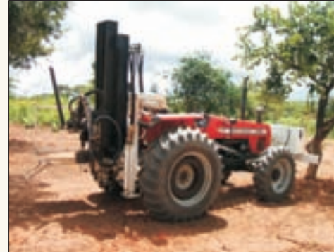
TRACTOR MOUNTED AUGER DRILL
