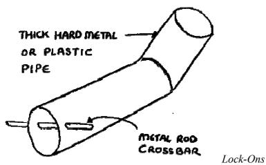
Concrete lock-ons, also called "dragons", are an advancing technology. Set in chimney stacks, in houses, up trees, at the base of trees, in oil barrels, in roads, in cars (immobilised or still drivable) and in tunnels, they have delayed evictions by days. Mobile lock-ons pose a real threat to free flowing infrastructure systems...
