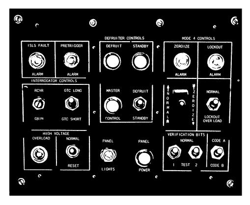
Figure 3-5.—Control monitor front panel.
