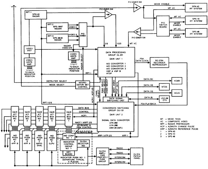
Figure 3-7.—CATCC DAIR system interlace block diagram.
