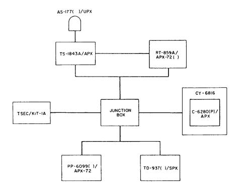
Figure 3-6.—Typical shipboard Mark XII transponder section.
