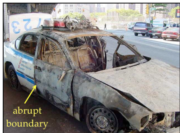
Fig. 25 - Police cruiser with unusual damage pattern.
