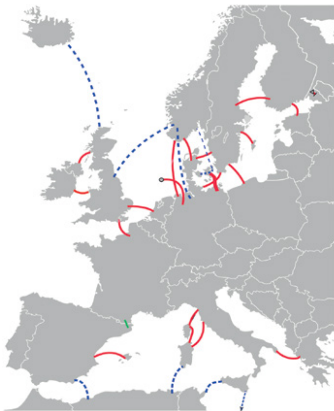
FIGURE 20 Existing and proposed interconnections of High Voltage Direct Current (HVDC) power cables across the European continent 36 . Red: existing, green: approved, blue: under consideration.
