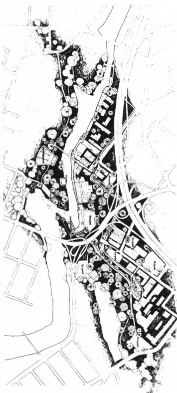
A detail of an 1877 map (left) shows the raceway in its final form. The Urban Deadline drawing (above) shows the same area after the loop of Interstate Highway 20 has been built (late 1970s). This route—which saw off a corner of the oldest part of Paterson—has been chosen for reasons which include the following two: 1) low density of the industrial district, and 2) lack of opposition from the adjacent residential district, which is to say, the poor will put up with it. Urban Deadline chose the site for the center of a renewal proposal because 1) it is the heart of Paterson's history, and 2) its development may neutralize the effect of the highway and prevent a poor section of the city from becoming another Watts.
