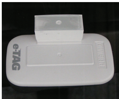
FIG4 Sydney, Australia's, Cross City Tunnel e-tag. The Cross City Tunnel is a fully electronic toll road, and there are no toll booths for cash payment. As the vehicle passes one of the tolling points of the tunnel, the tag will transmit a signal to the toll gantry. This acknowledges and deducts the appropriate toll amount from one's toll account. (Photo courtesy of Jason Sargent.)
