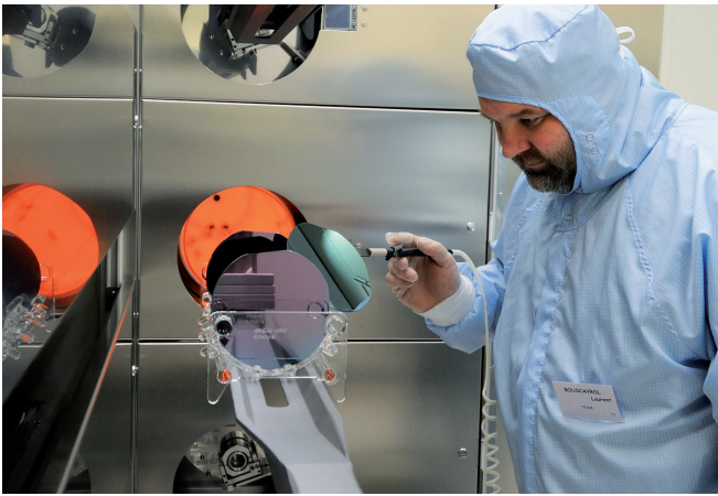
Micro- and nanotechnologies platform: automated oven for the growth and deposition of silicon-based materials.
