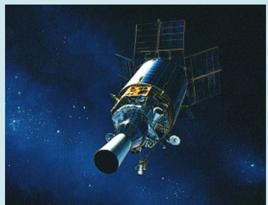
Figure 3. Nuclear Detonation Detection payloads are provided on both the global positioning system navigational satellites (left) and the Defense Support Program early launch detection satellites (right) .
