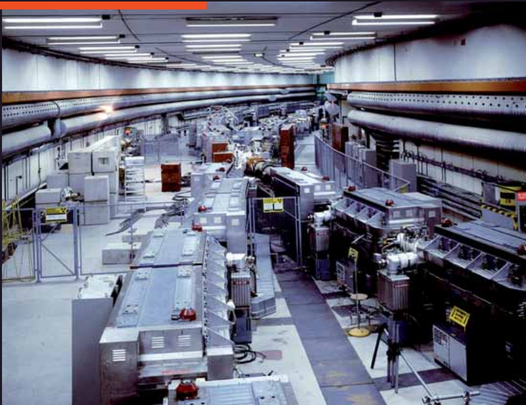
7. The Intersecting Storage Rings (ISR)—the first proton collider in the world—operated between 1971 and 1989. Made up of two identical 300-meter rings that intersect at 8 points, the machine, whose beams were supplied by the Proton Synchrotron (PS), helped provide hints that protons were composed of smaller parts.
