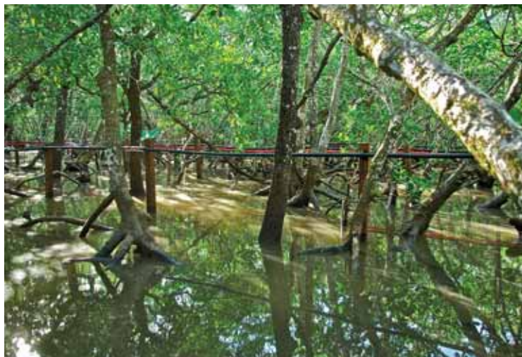
▲ In Mayotte, the experimental plot of mangroves ( Rhizophora mucronata ) is criss-crossed by a network of pipes that release wastewater under controlled conditions.
