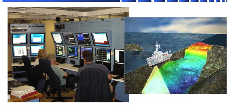
Multi-beam Echo-sounder: Determining broader area bathymetry and detecting targets of interest
