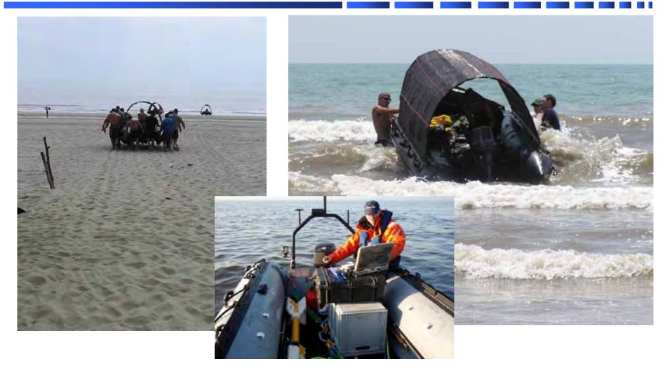
Shore-based or Ship-based Small Boat Team: Lightweight, Short-Distance Range, Portable, Maneuverable, Working Depths 5-100 ft
