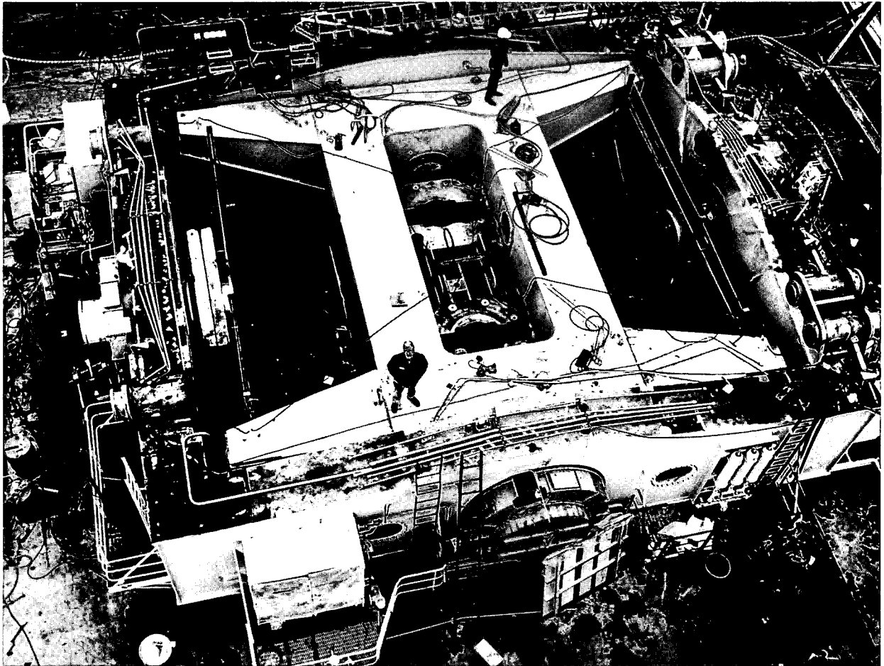
Figure 13. Inner and outer gimbals which removed the roll and pitch motion
