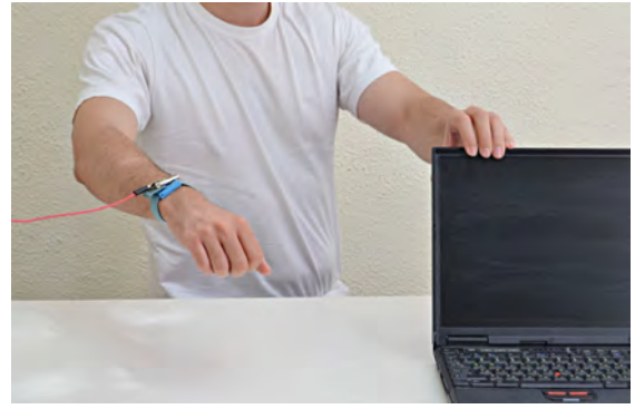
(b) Adaptive “human touch” attack by bare hand. The wristband is connected to the probe wire.
