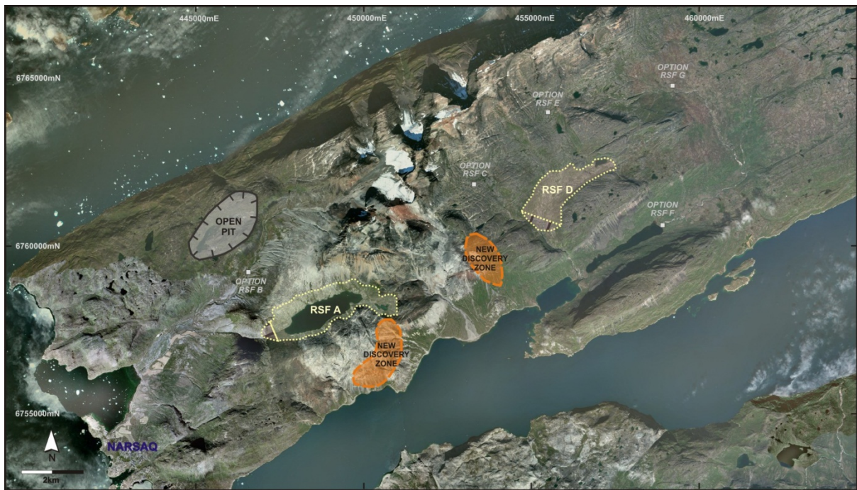
Figure 2.7.1 Residue Storage Facility Location Options
