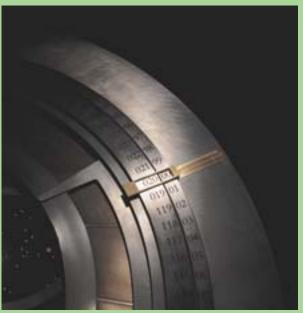
10,000-YEAR CLOCK under development by the Long Now Foundation will be strictly mechanical. Like the first prototype of the clock (top), the final, monument-size version will probably use a torsional pendulum to count minutes but will display only the current year, century and millennium (bottom).
