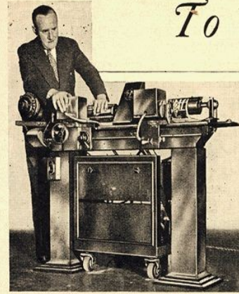
Three-color printing plates, which take 36 hours to produce by man-power, are turned out in 30 minutes by this electric machine.
