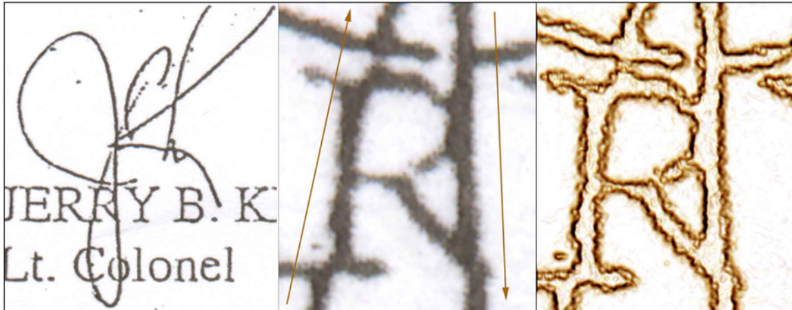
Figure 10: Left: Killian signature block taken from a questioned 01 August 1972 memo at approximately 6X. Center: “R” with accompanying line alleged to be from Killian’s signature blown up to permit microscopic examination. Note: brown arrows indicate direction of signature strokes. Right: Same view of the “R” and line using 3D visualization.
