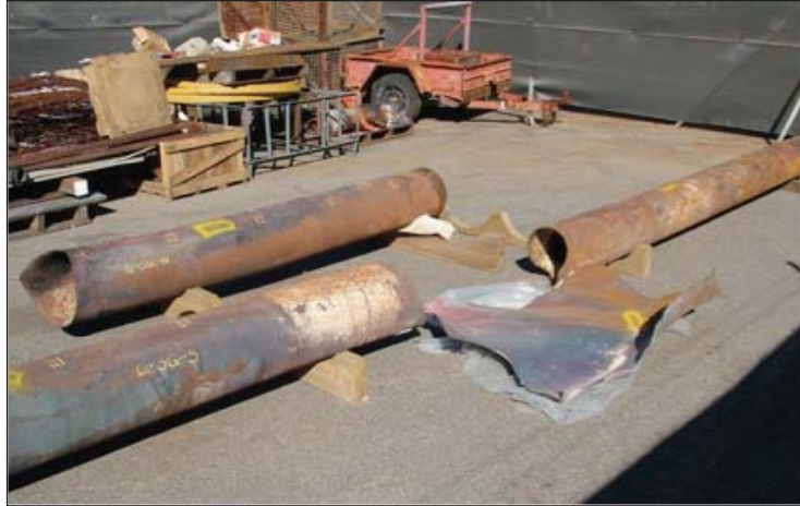
Figure 2: 12 Sales Gas Pipe sections (12-SG-S, 12-SG-N & 12-SG-N-FE) and 12 Sinbad / Campbell Pipe section (12-SBC-N) laid out in similar positions as to that as removed from the Varanus Island site (Pearl Street Report 8A5/MET 9, Appendix 1, Image 5)
