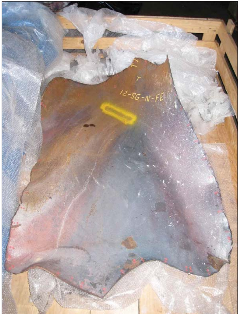
Figure 3.1.1 General view of the inner surface of the 12-SG-N-FE piece of pipe, unwrapped by bursting
