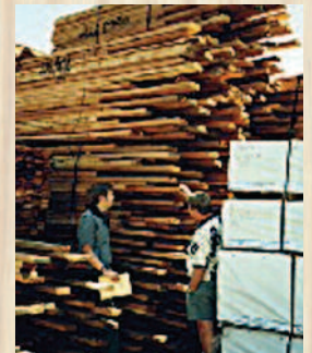
Our partner mills supply us with miles of 401 clear grade roughcut stock.
