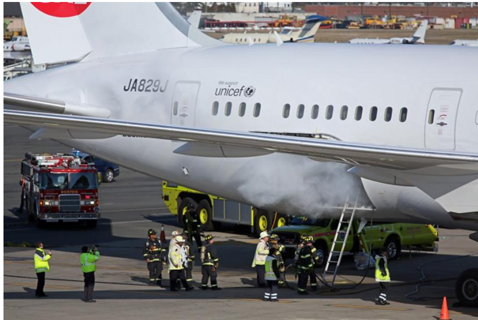
Figure 1. Smoke emanating from the aft electronic equipment bay.
