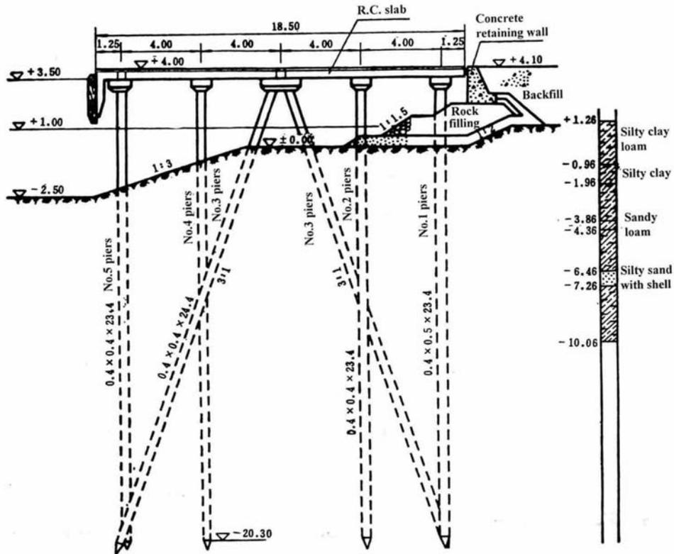
Figure 2. Cross section of the Xinhe external transport terminal (in m).
