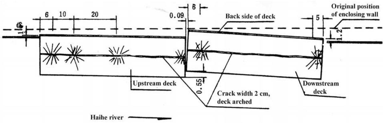
Figure 4. A sketch of damage to the Xinhe external transport terminal (in m).
