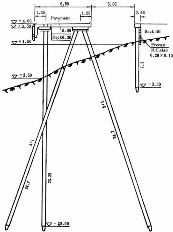
Figure 9. Cross section of the Frontier Station Pier (in m).
