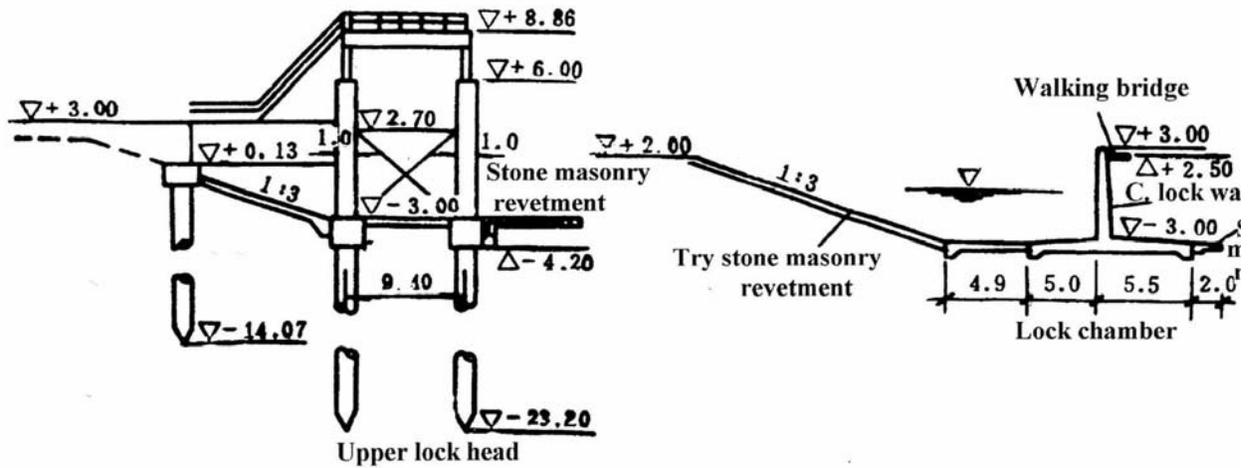
Figure 11. Sectional drawing of the Peizhuang ship lock (in m).
