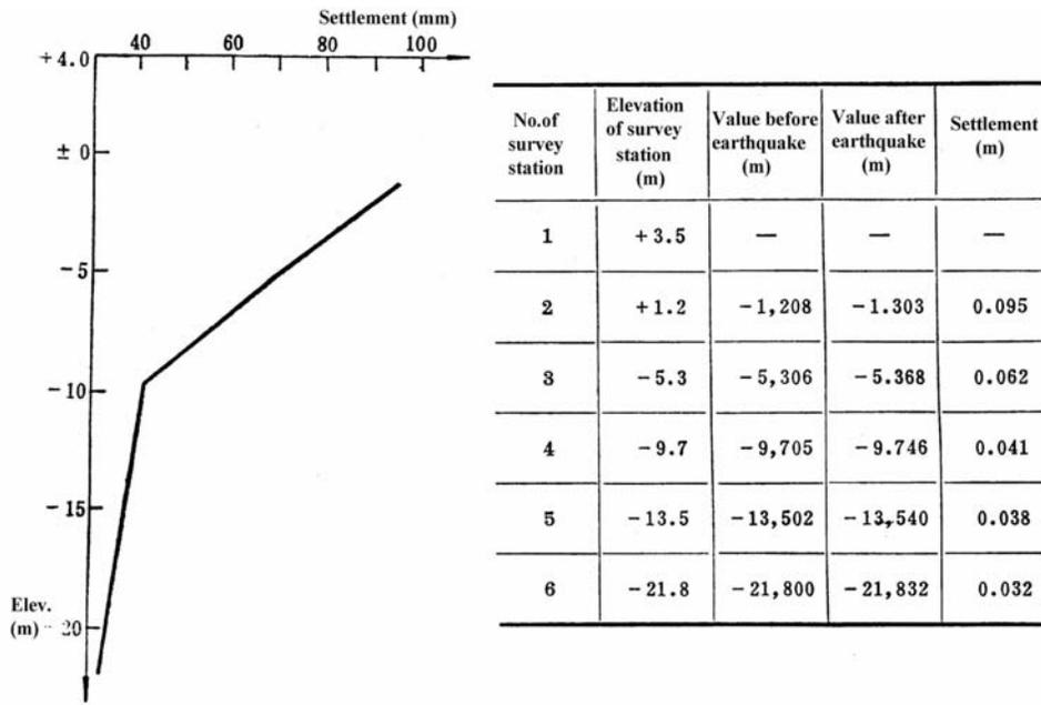
Figure 7. Curve of settlement at the sand drain test area.
