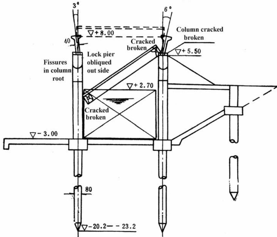
Figure 12. A sketch of the damage to the upper lock head at the Peizhuang ship lock (in cm).
