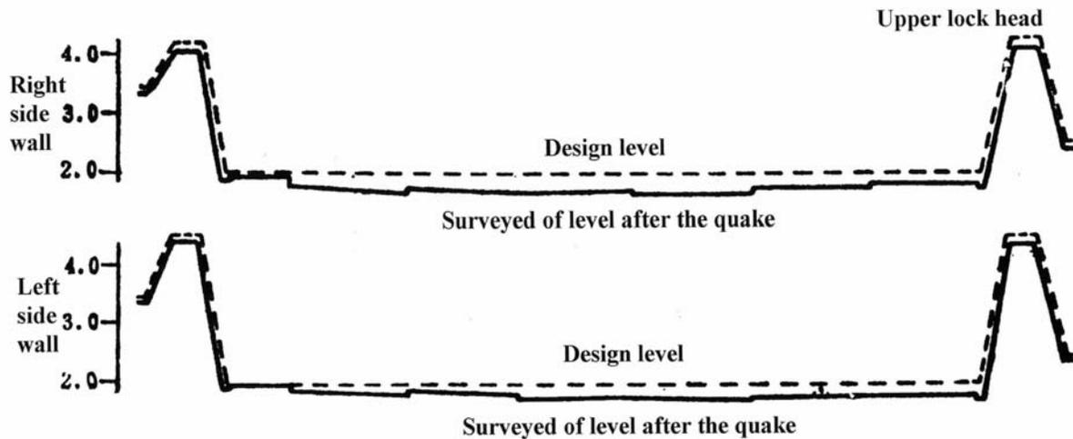
Figure 6. Settlement of the top level of the lock wall at the Beitang ship lock after the earthquake (in m). (Surveyed level after the earthquake is based on the datum horizon point that had been settled 0.62 m)
