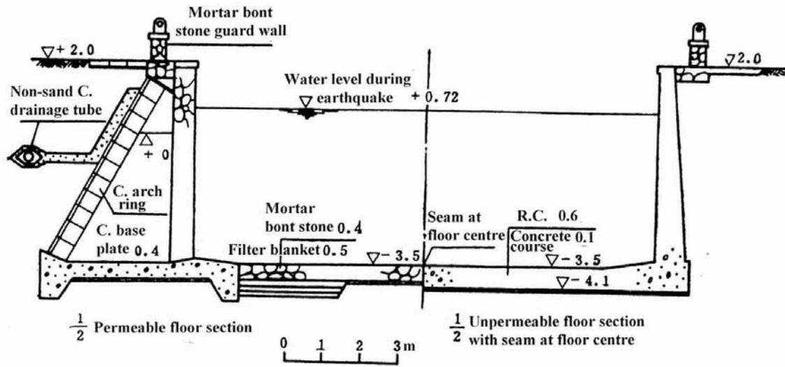
Figure 5. Lock chamber sectional drawing of the Beitang ship lock (in m).
