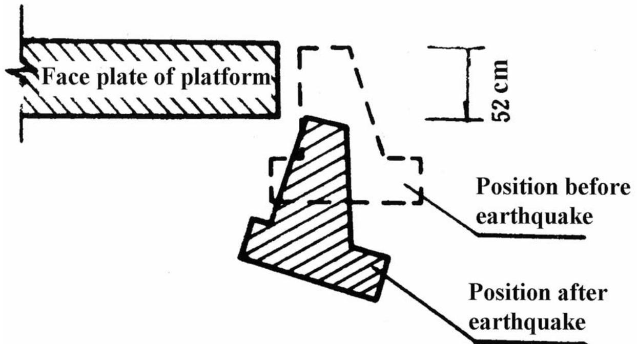
Figure 12. A sketch of a map showing the settlement of a retaining wall after the earthquake.
