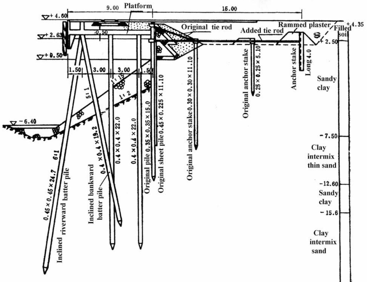
Figure 11. Cross section of the No. 9 wharf (in m).
