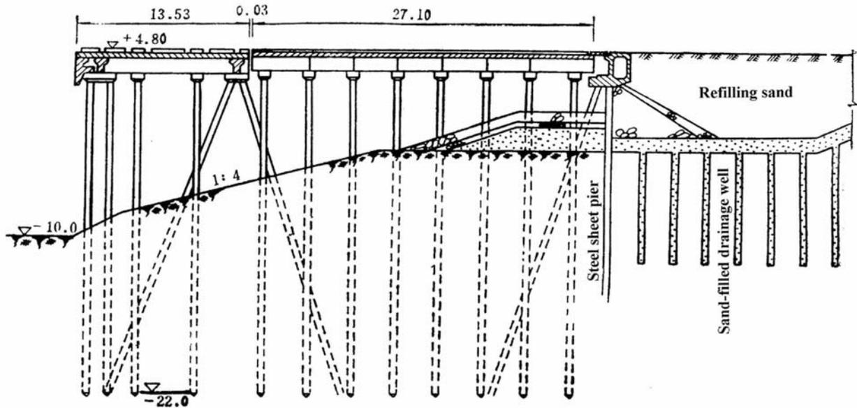
Figure 10. Cross section of No. 9-No. 13 berths at the New Port of Tianjin (in m).
