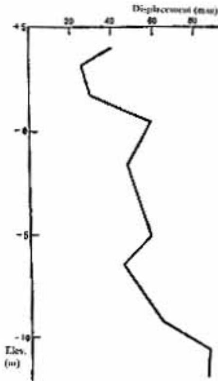
Figure 8. Curve of soil layer displacement at sand drain test area.
