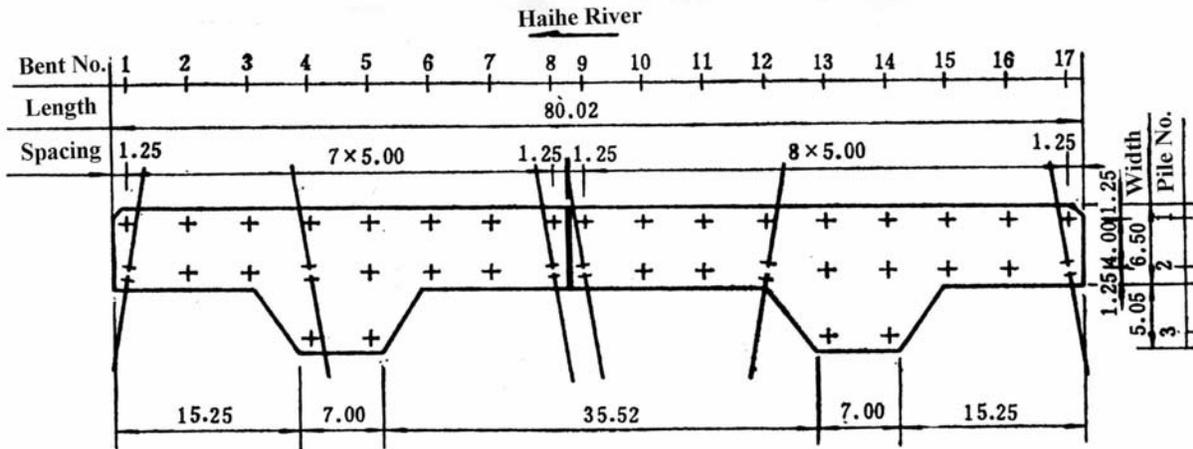
Figure 8. Plan of the Frontier Station Pier layout.
