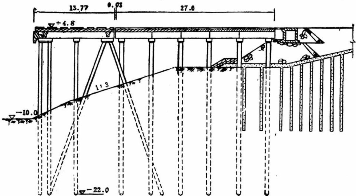
Figure 11. Cross section of No. 22-No. 24 berths at the New Port of Tianjin (in m).
