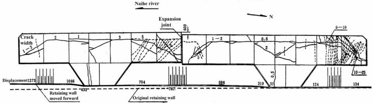
Figure 10. State of pier displacements and cracks of pier decking at the FIS pier (in mm).
