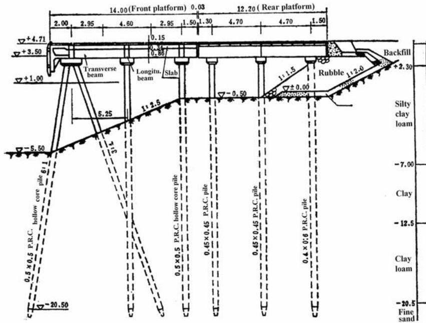
Figure 12. Cross section of the No. 10 wharf (in m).
