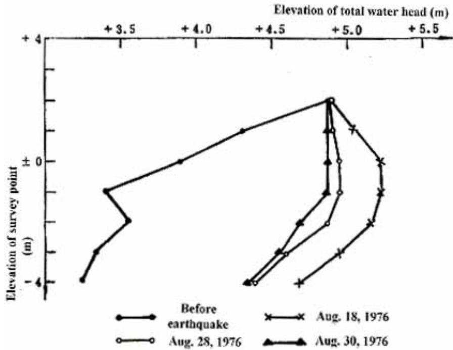
Figure 9. Surveyed results of the ground pore water pressure at the sand drain test area before and after the earthquake.
