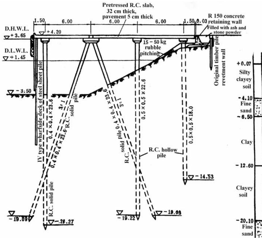
Figure 7. Cross section of the Yujiapu foreign trade terminal (in m).
