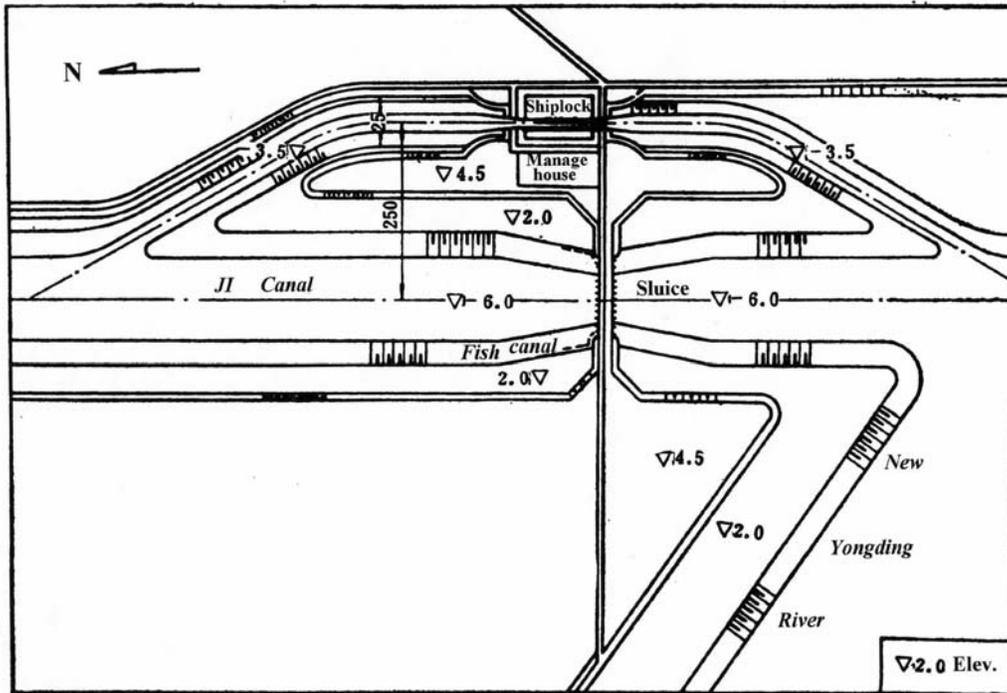
Figure 2. The Beitang water conservancy project layout plan.
