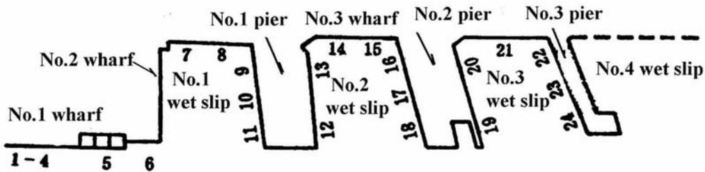
Figure 6. Arrangement plan of berths of the New Port of Tianjin.
