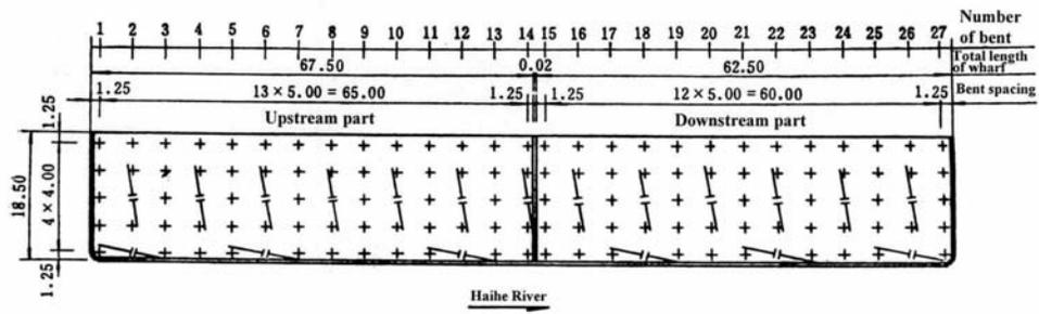
Figure 3. Pile layout of the Xinhe external transport terminal (in m).
