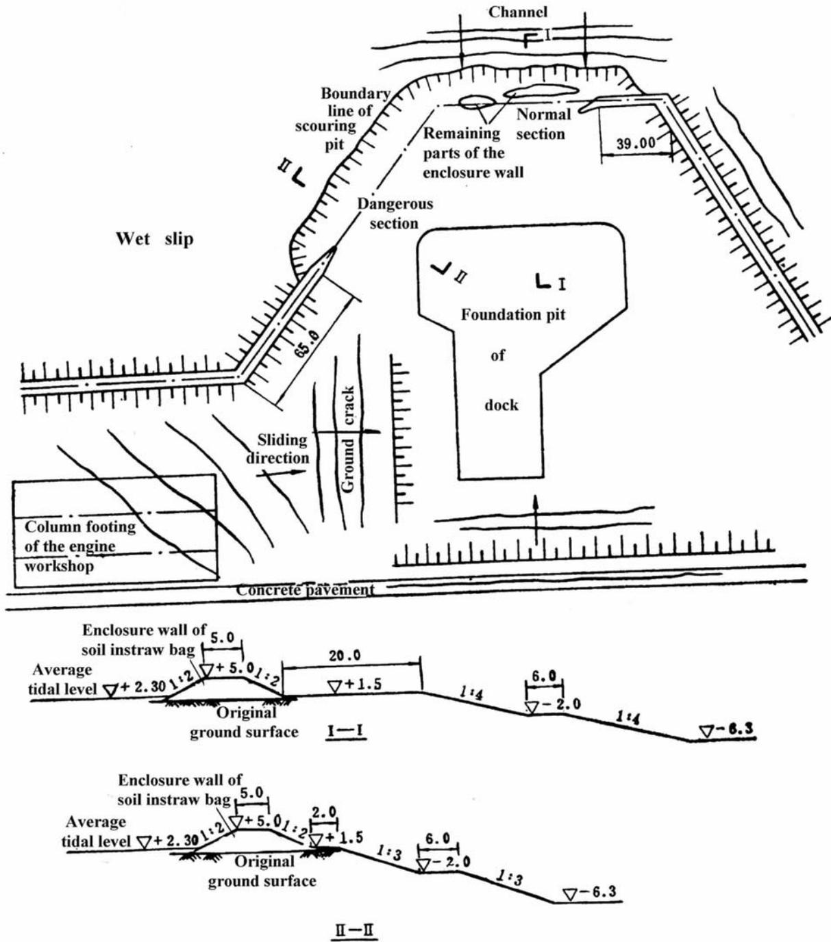
Figure 5. Plan sketch map of earthquake hazards damage to the enclosure wall and foundation pit of the dock for the Marine Petroleum Exploration Bureau.
