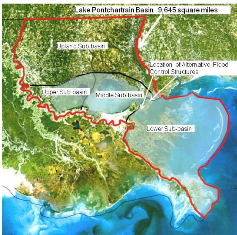
Figure 7: Lake Pontchartrain Basin (red outline), and the estuary sub-basins. Shaded area is approximate area of the estuary. Alternative Flood Control structures at the tidal passes would be positioned with \frac{1}{4} of the estuary on the protected side and \frac{3}{4} of the estuary on the flood side.
