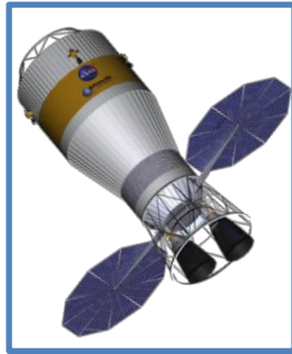
Cryogenic Propulsion Stage (CPS)
