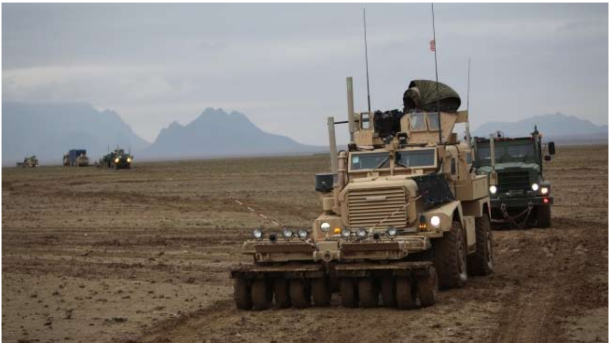
MRAP pushes a mine roller through the route ensuring the path is clear of IEDs during a 5-day convoy to FOB Edinburgh, Afghanistan.
