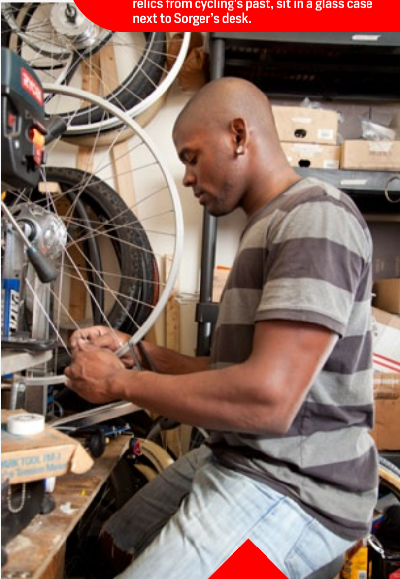
An employee hand drills each Swift wheel and adds the spokes in DBC's back room.
