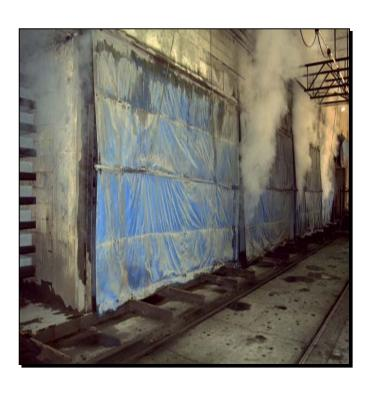
Block remain in the kilns for 24 hours. They are baked in a moist steam heat at 140 degrees Fahrenheit.
