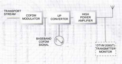
A typical digital transmitter set-up.
